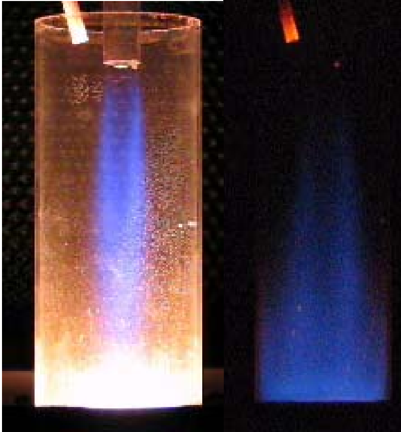
Figure 7. Photographs of the SPRF combustor flame emission when operating premixed at an equivalence ratios of: 0.74 (left) and 0.55 (right).
